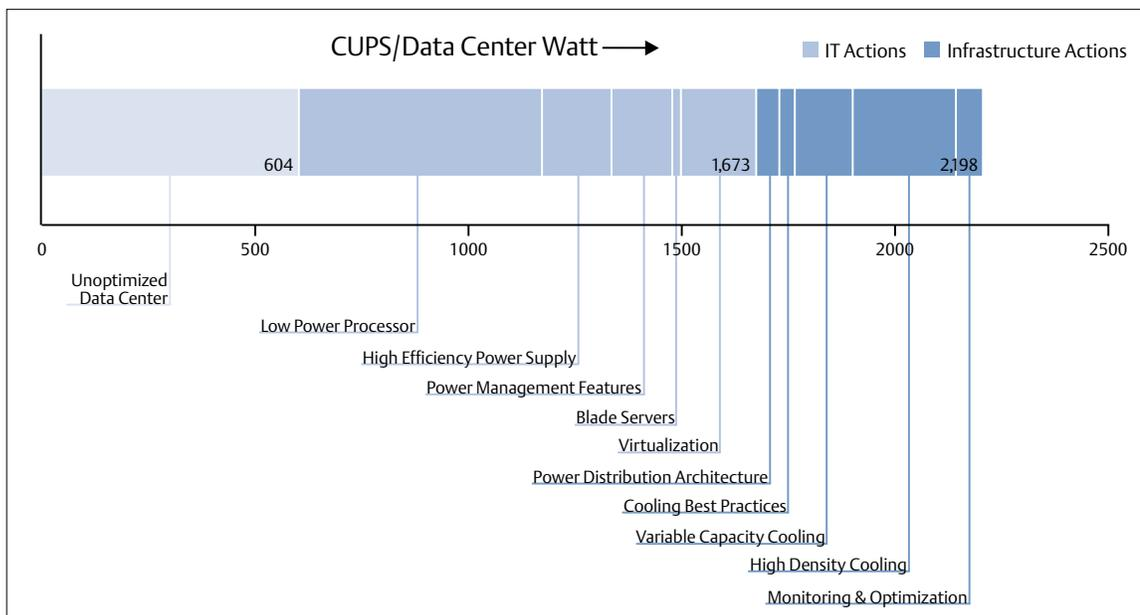
**Figure 9.** Prior to any enhancements the model data center was able to produce approximately 604 CUPS/watt. The Energy Logic roadmap increased efficiency to 2198 CUPS/watt (3.6x) with the largest increase in efficiency being delivered by adoption of low power processors.
