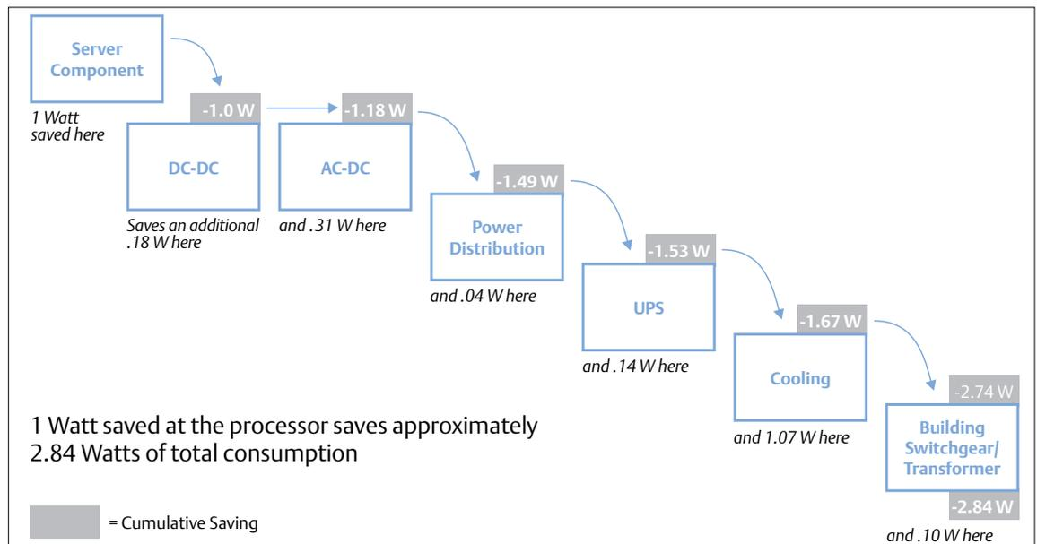
**Figure 1.** Energy Logic demonstrated how savings at the server component level cascade across supporting systems, increasing their impact.
